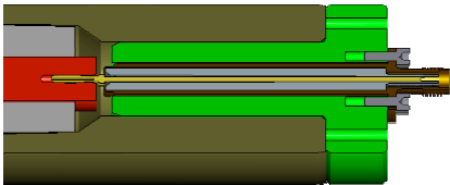
Coaxial SMA connector press-fitted into the customers housing
