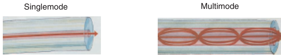
Figure 2. Singlemode and Multimode Fibers
